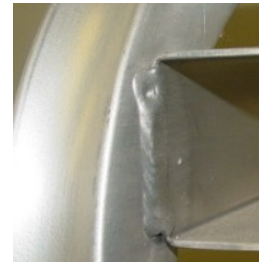
Robotic MIG Welded Shelves and Frames
